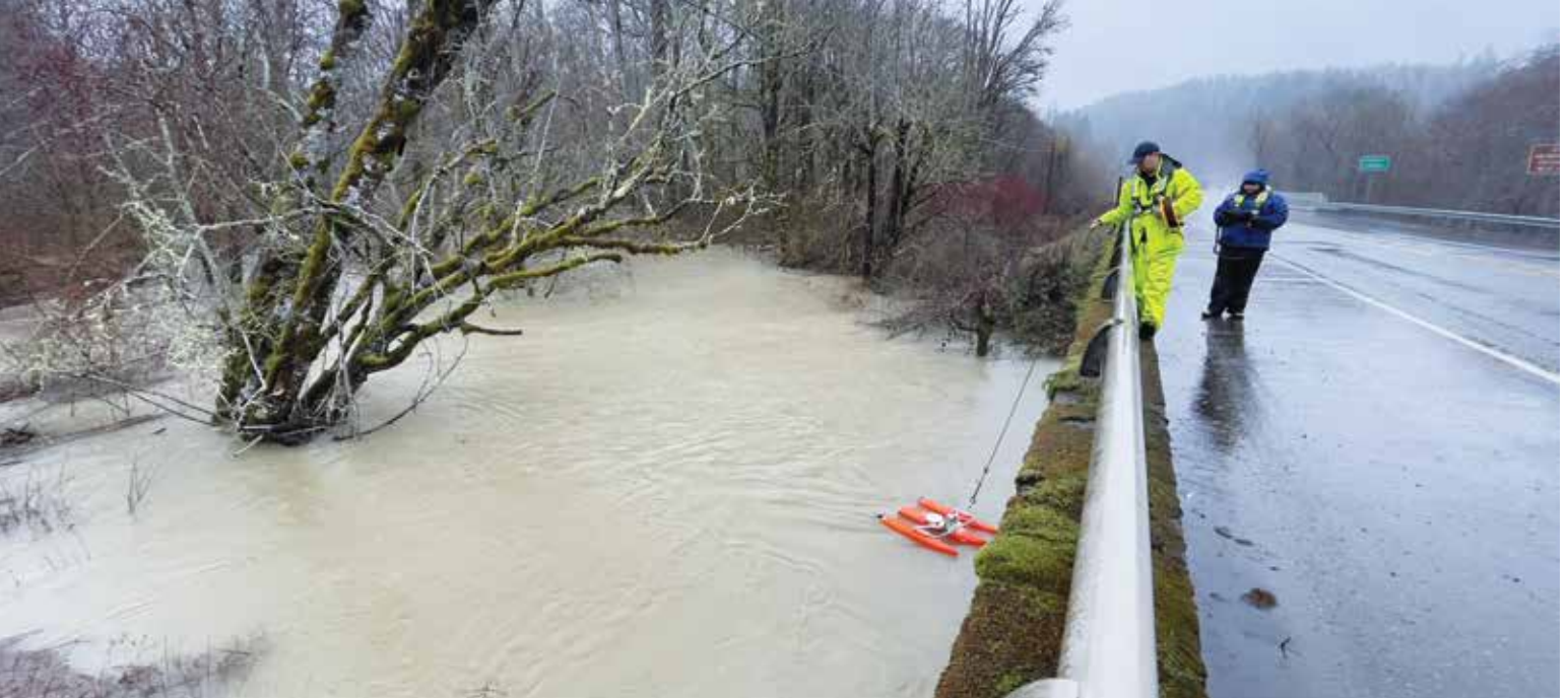
Above: USGS hydrological technicians Andy Cripps and Fred Reed collect flood flow measurements off the Weaver Creek bridge during a recent heavy rains in the Skokomish watershed. Below: Skokomish Tribe environmental biologist Julian Sammons reads the river stage height from a gage in a Skokomish River tributary under Highway 101. Photos: Tiffany Royal
