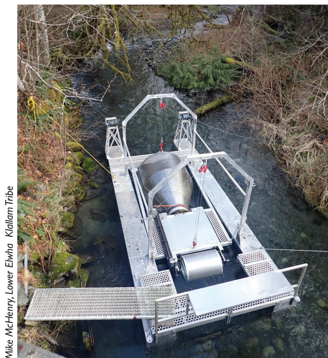
A smolt trap on Little River (one of three within the Elwha River valley).
