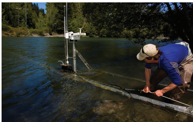
Setting up SONAR camera for enumeration of adults.
